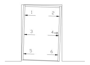
**2a.** Align and grip the doorset in the opening, using external packings.
