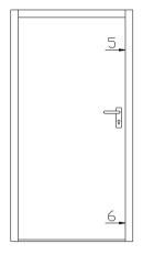
**6**. Close the door again, then fit the last 2 fixings into face 5 of the lock jamb.
