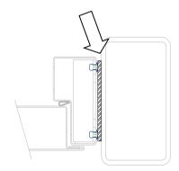
2b. Fitting external packings between the jambs and the structural opening.
