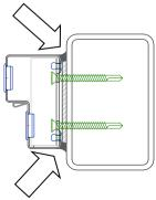
12. Apply mastic or flashings to seal frame to building. Fit blanking plugs to the frame fix access holes.
