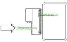
7. Open the door again, then second fix through the access holes in the frame reveals.
